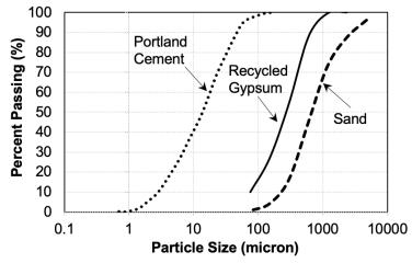
Figure 1. Particle size distribution of gypsum, sand and Portland cement. Note: Portland cement data retrieved from Sata et al. [21]
