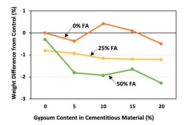
Figure 8. Difference of specimens' weight in comparison to control mix on day 5
