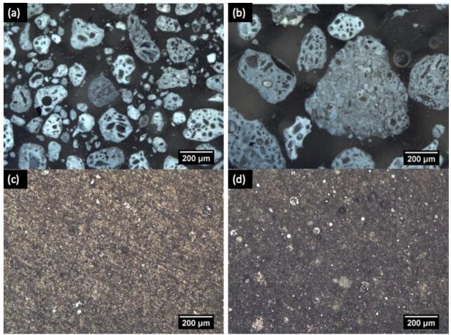
Figure 3. Magnified view of (a) fine gypsum; (b) coarse gypsum; (c) cement; (d) fly ash
