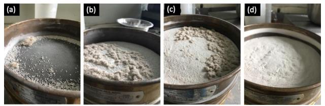
Figure 2. Gypsum retained on sieves (a) No. 16; (b) No. 30; (c) No. 50; (d) No. 100
