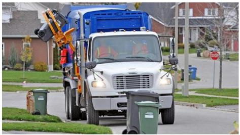
Photo 3 – Photo of a fully automated cart-based waste collection truck from the City of Guelph. Source: Guelph Mercury file photo
