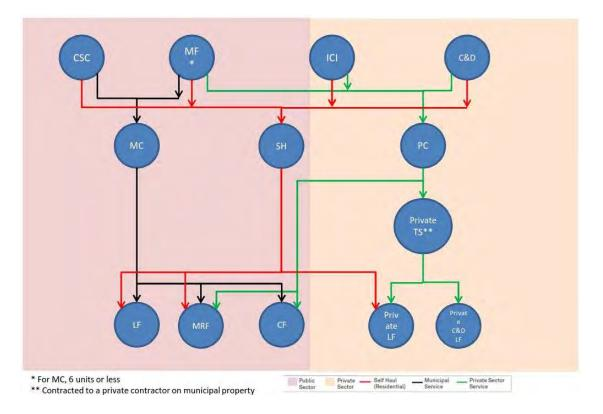
Halifax contracts for the operation of two privately owned compost plants, each with a capacity of 25,000 tonnes, operation of 36,000 tonne capacity Materials Recovery Facility (MRF) owned by HRM and municipally owned waste processing and disposal facility (landfill) and a transfer station jointly operated by HRM and the landfill contracted operator. These facilities process materials from HRM residents and the ICI (Industrial, Commercial, and Institutional) Sector.
