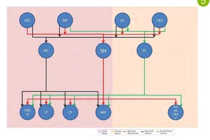
A flow diagram illustrates the solid waste management system. Shading is used to identify the various aspects of the solid waste system that are controlled or managed by the subject community. It also identifies other parts of the solid waste management system that are controlled by the private sector or other public sector entities.
